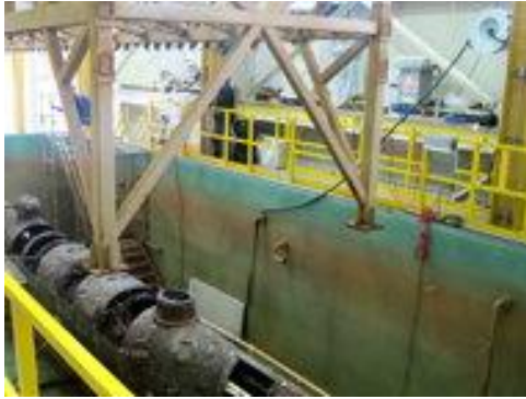
A steel truss that had surrounded the Confederate submarine H.L. Hunley is raised ...
